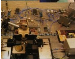
ME inhouse developed harmonic load-pull set-up
